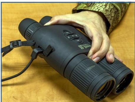
Insert the USB type C plug in to the USB type C media port.
