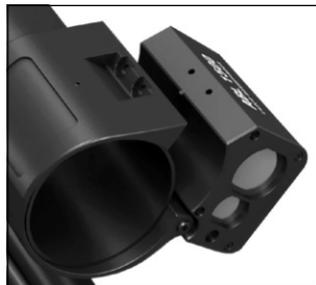
Unscrew the two Allen screws from the ABL housing and open the latch. Slide the ABL housing with the latch open over the threaded sleeve, and remove the housing from the sleeve. Use a few drops of lubricant oil on the threads before attaching the adapter ring
