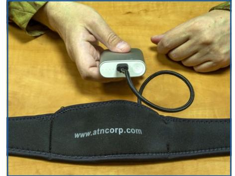
Once the battery has been activated, place it in the provided battery compartment in the center of the Neck/Shoulder strap and close the zipper.
