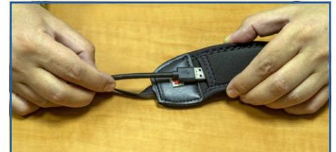
Pull the cable all the way through until it reaches the center of the Neck/Shoulder strap battery holder compartment.
