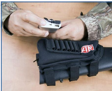
Place the battery with the USB cable attached in to the rifle pouch battery compartment.
