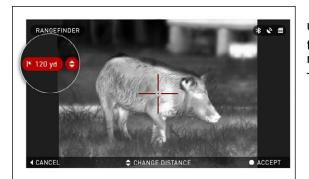
Change distance value using UP and DOWN buttons . To accept the new distance, press ENTER button ...
