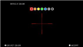
Movement between the colors is carried out using the LEFT and RIGHT buttons . Then press ENTER button to accept your color.
